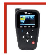
The Trigger tool is the perfect device for the person in charge of confirming tire pressure and temperature as the car/moto leaves or enters the pits and after the tire mounting process.
