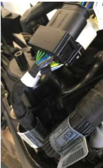
Image 5: Upper / lower engine loom on RHS of airbox.
