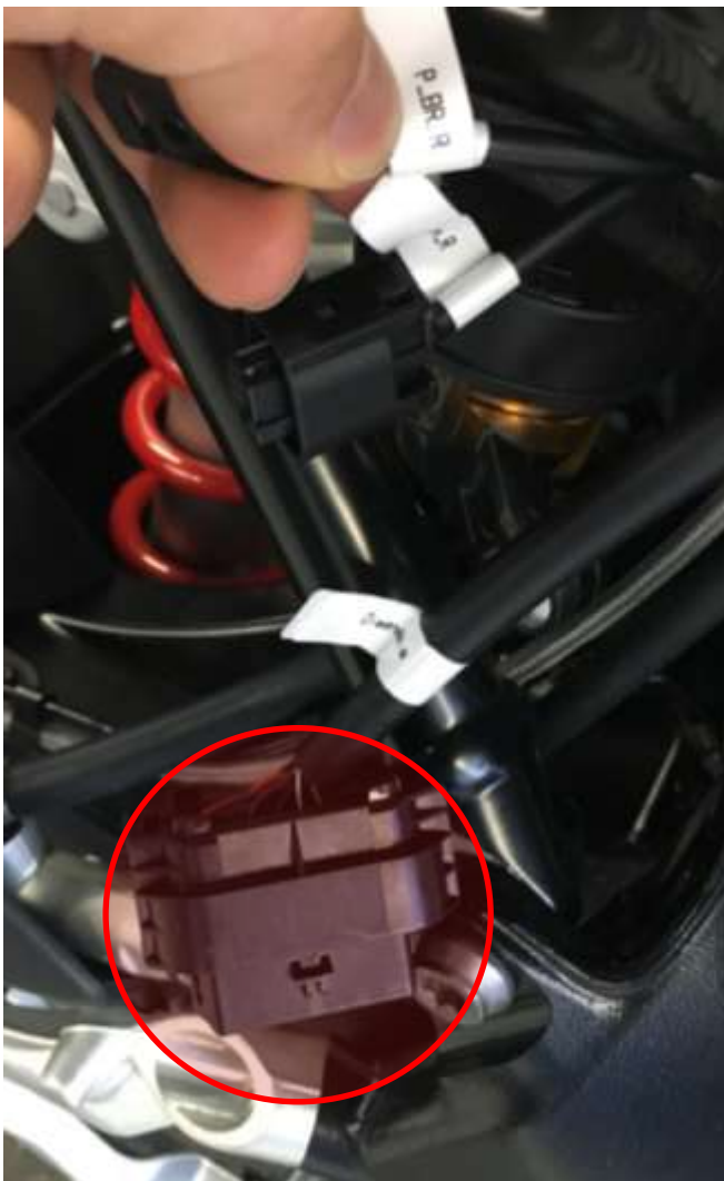
Image 18: Rear sensor interfaces, diagnostic connector.
