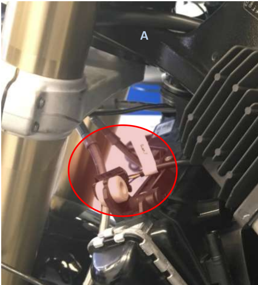
Image 11: Front suspension sensor location.
