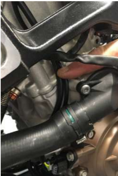
Image 10: Leads away from header pipes.
