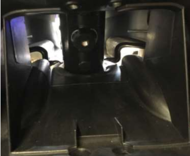
Image 1: Intake air duct without air flap.
