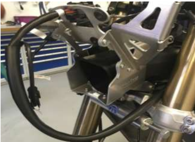
Image 22: Front chassis loom on RHS of intake air duct.
