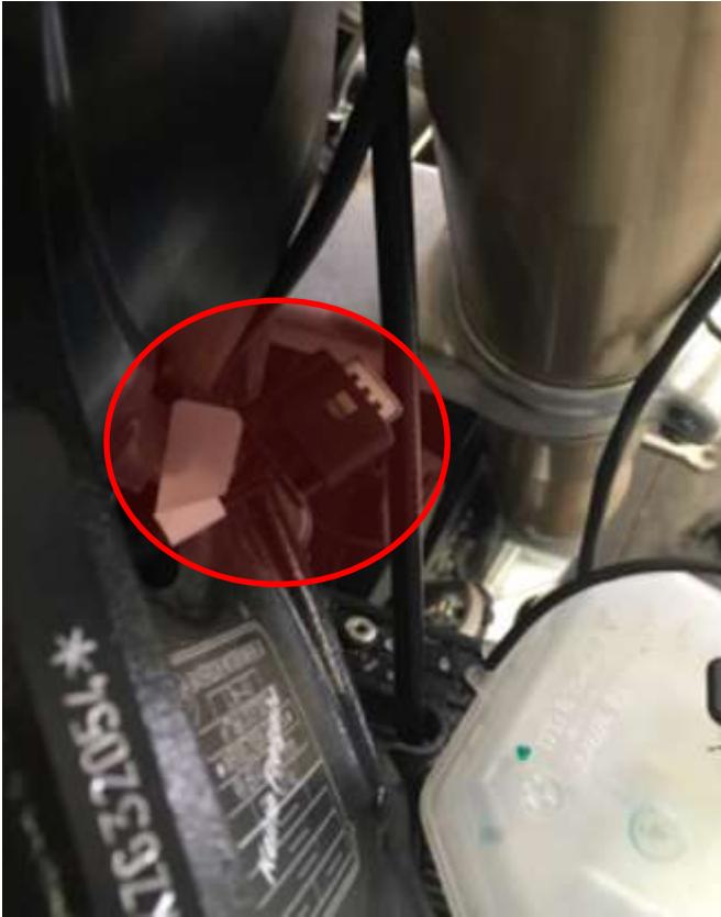
Image 12: Front brake pressure sensor connector around RHS fork leg.
