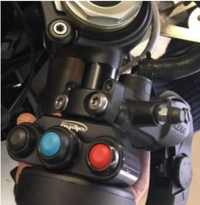
Image 27: RHS switch unit between throttle grip and brake pump.
