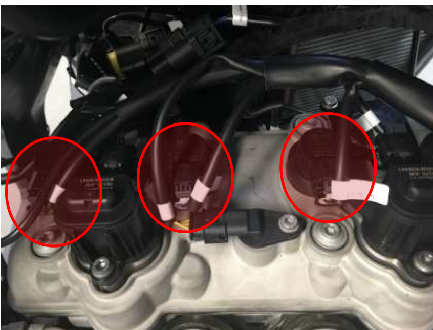
Image 2: Rotated ignition coils (all 4 coils must be rotated).
