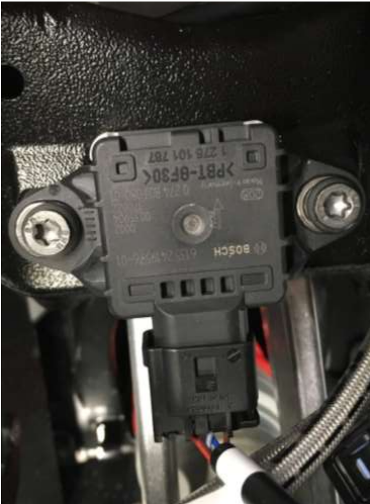
Image 31: Lean angle sensor facing to the rear end of the bike.
