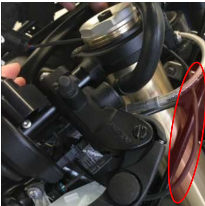
Image 26: Cable guidance of RHS switch unit.
