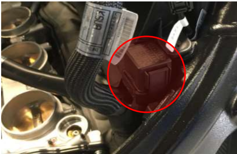
Image 13: Fuse box on RHS of airbox.
