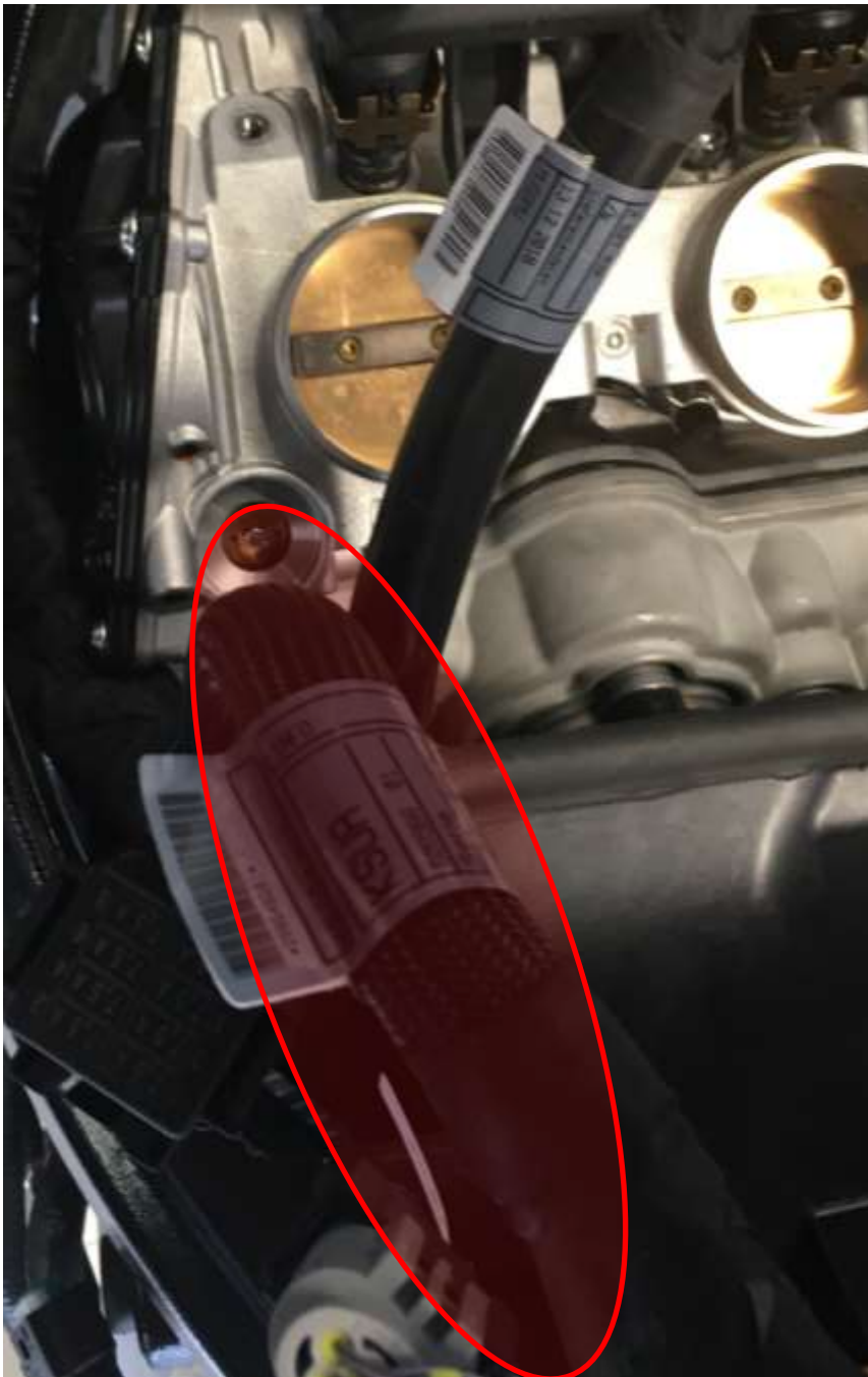
Image 7: Main strand of chassis loom down the RHS of the airbox and into RHS beam of main frame.
