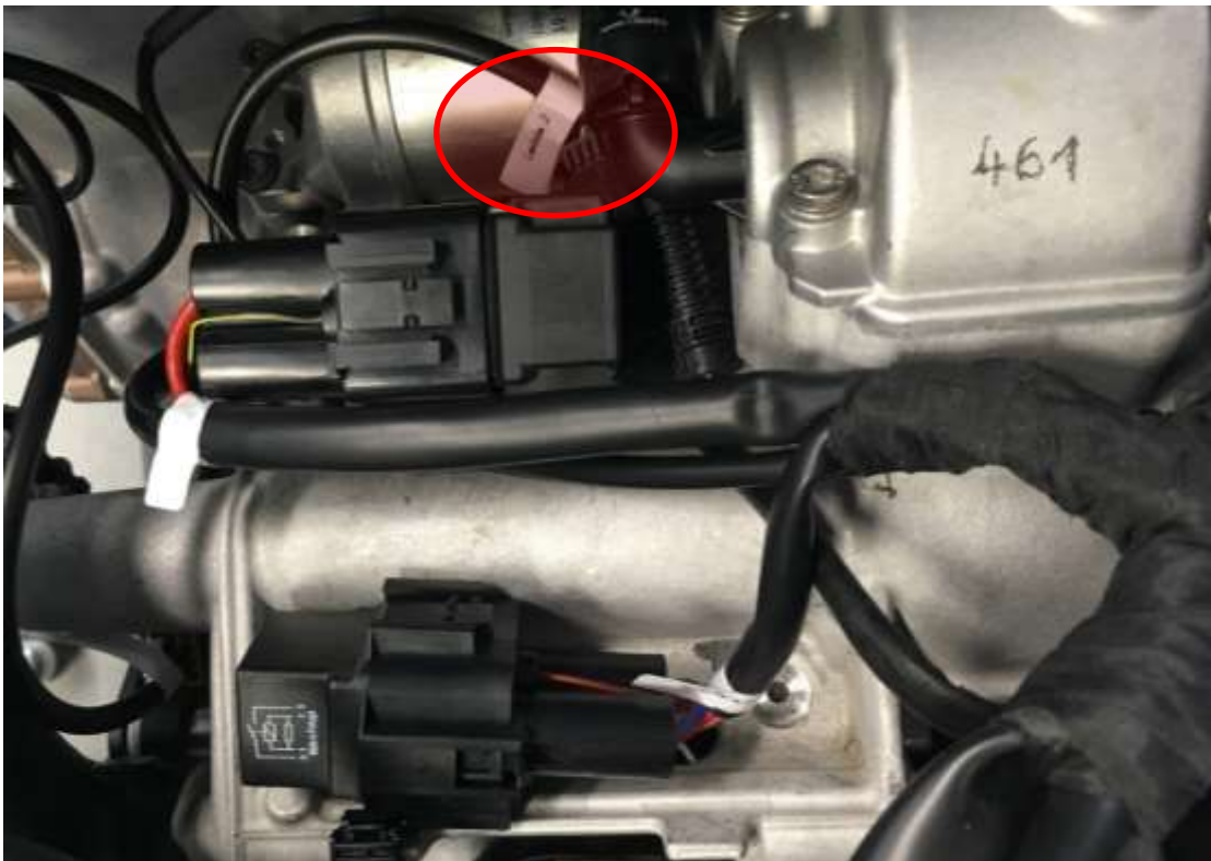
Image 17: Main-, starter-relay, and lambda connector behind starter motor.
