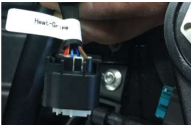
Image 29: Heat-Grips connector around headstock.
