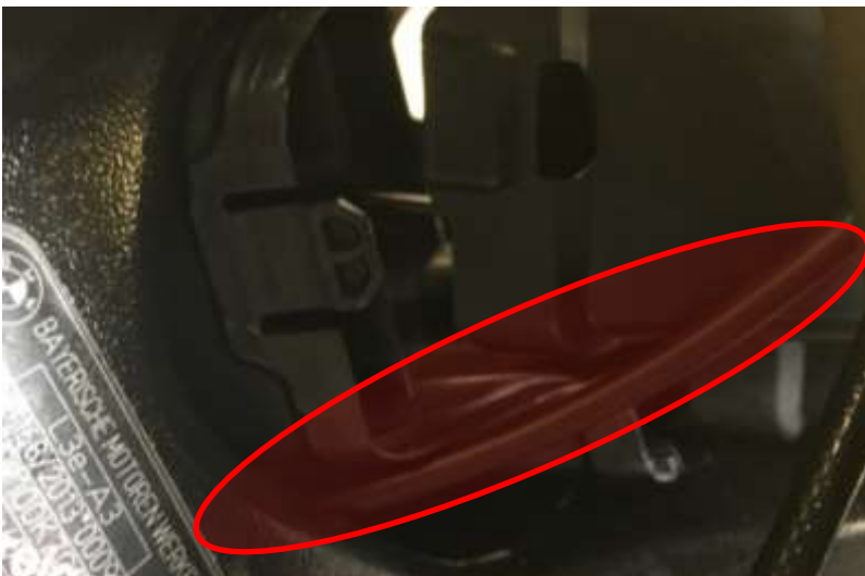
Image 24: Throttle grip module through RHS air intake duct.
