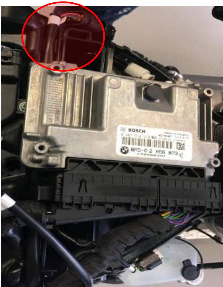
Image 6: Upper chassis loom on top of airbox.
