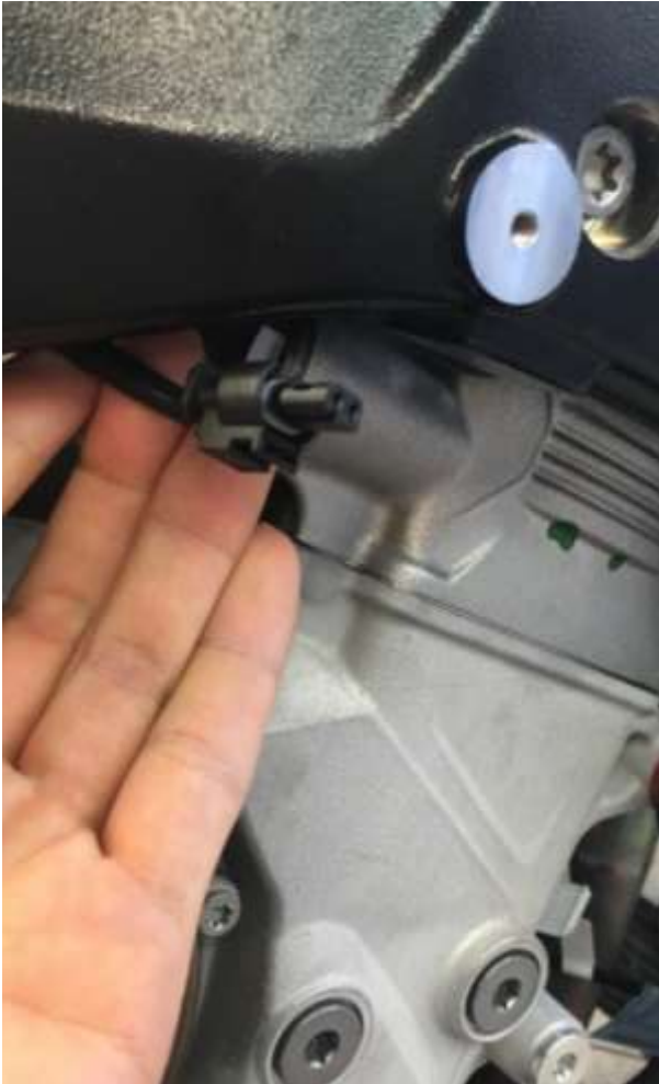
Image 15: 2-pin connector under RHS beam of main frame.
