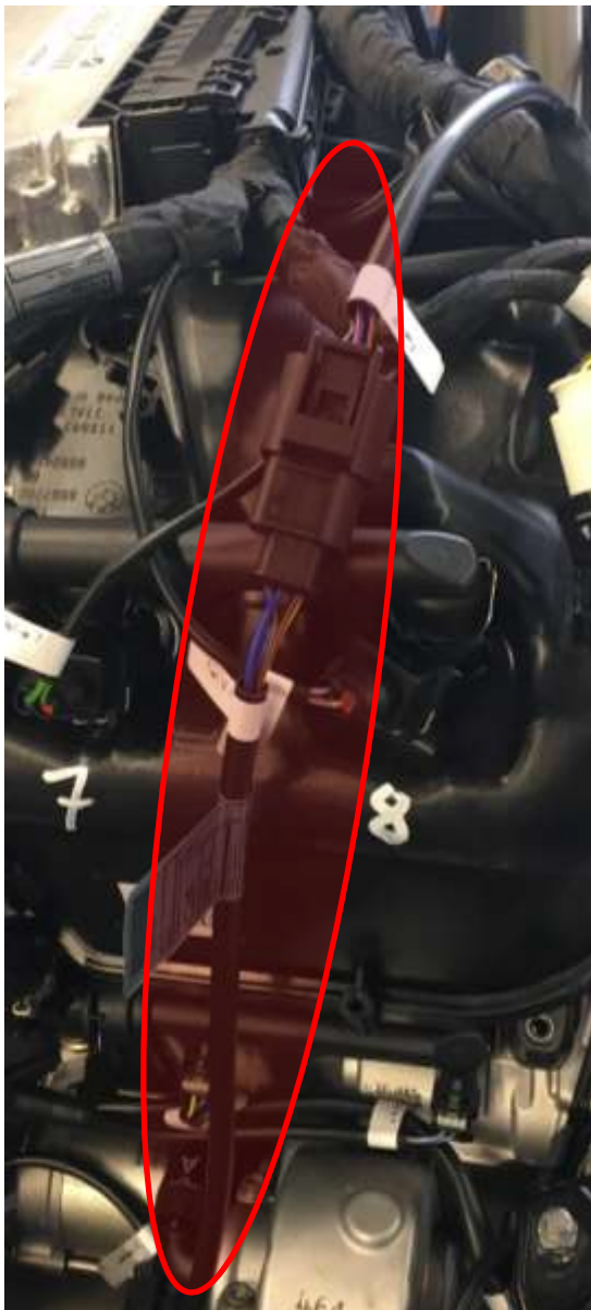
Image 25: Fuel chassis module behind airbox.
