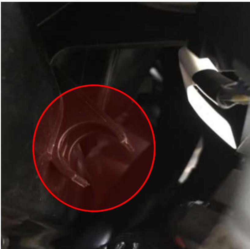
Image 14: RHS Airbox bracket to be removed.
