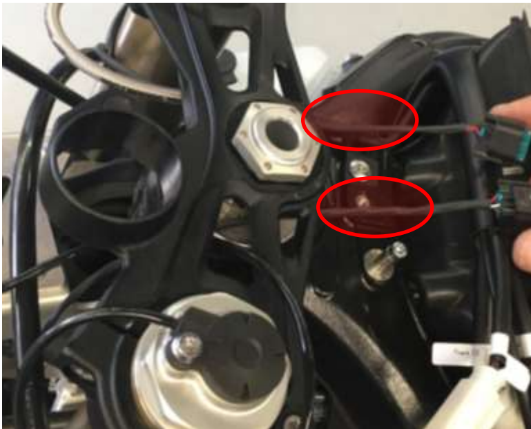
Image 28: Switch unit cables and their potential issues.
